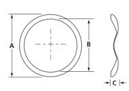
ullet Stainless steel spring washer for 15/32" (29 mm) mortise cylinder
